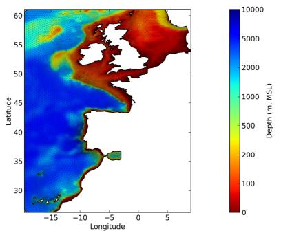
Fig. 1. Finite element grid and bathymetry.
