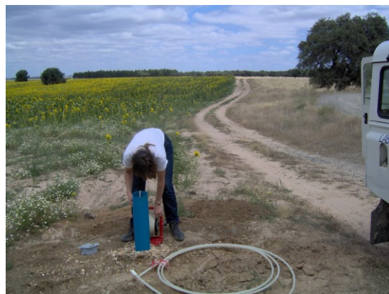
Fig. 4 - Piezometer for groundwater sampling
