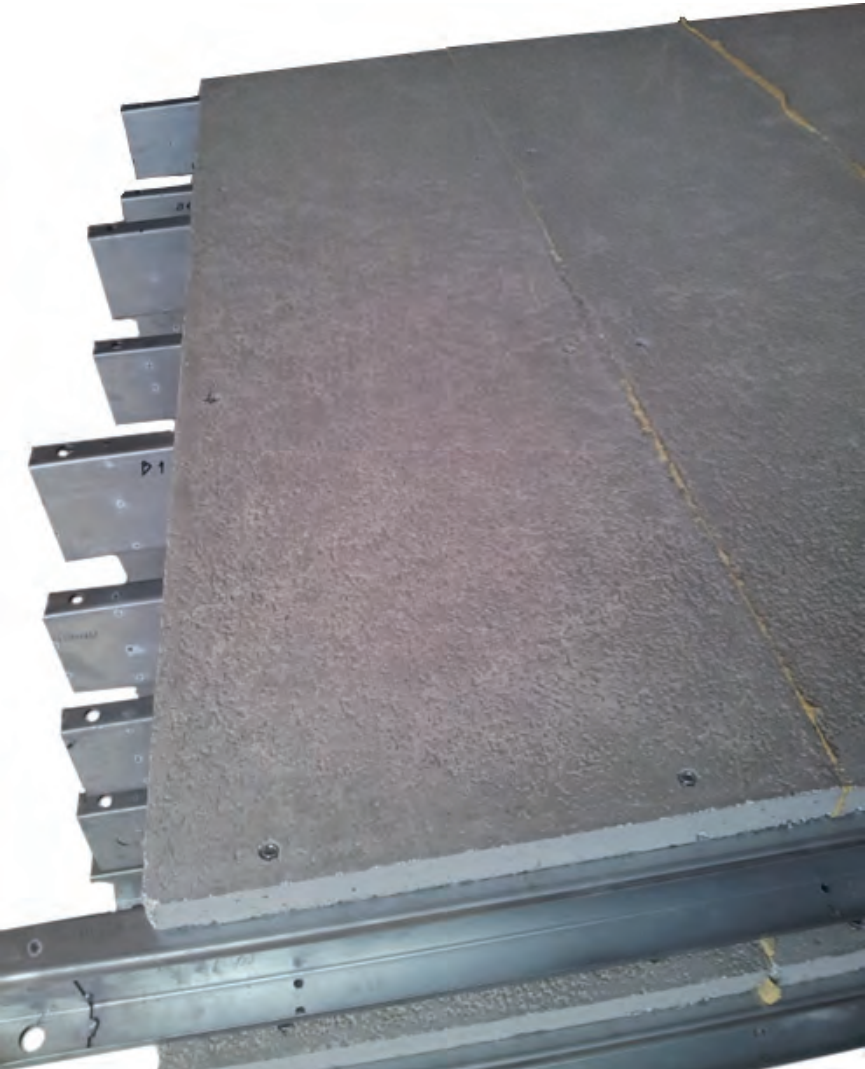
figure 2 | Panels evaluated in the test of the suitability of a corrosion protective system. Specimen detail after test and respective image analysis result.
