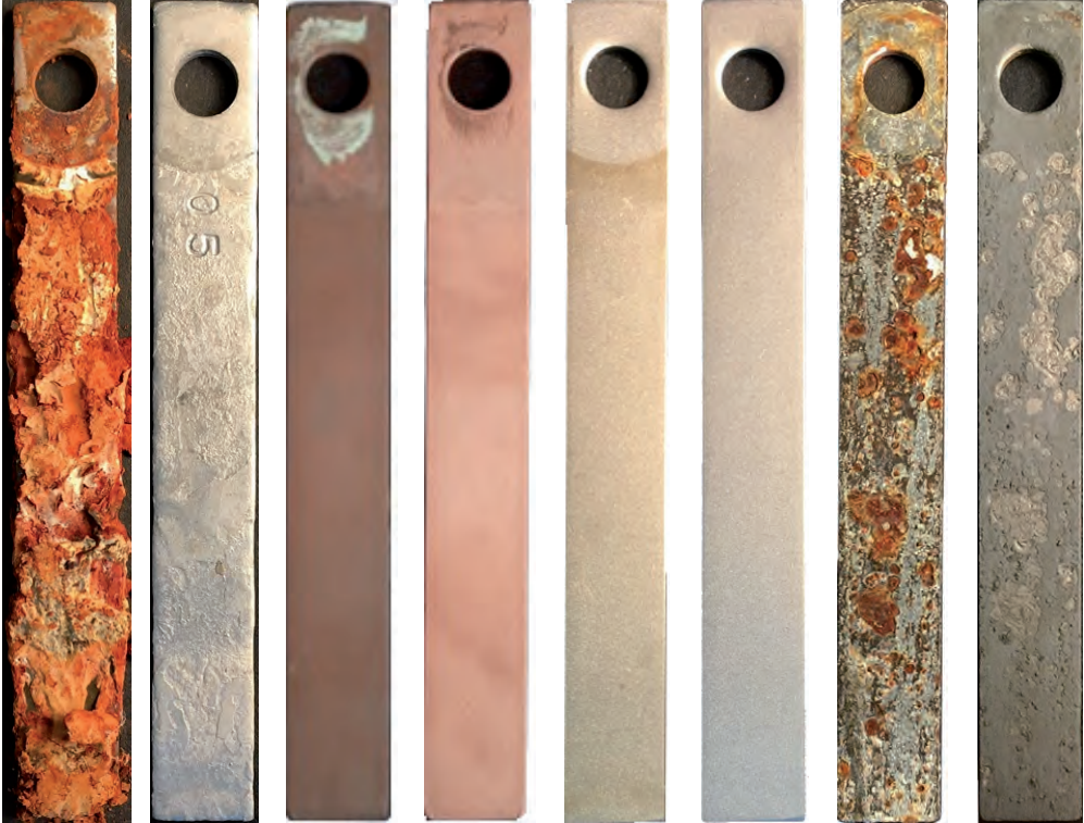
Carbon steel Copper Stainless steel Galvanized steel figure 1 | Metallic specimens assessed by the corrosivity of water test: left – after test; right – after chemical cleaning of the corrosion products.
