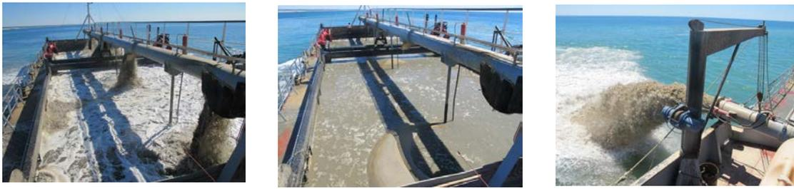
**Fig.2 – Different phases of the dredging operation: a) sediment pumping; b) full capacity tank; c) sediment injection**
