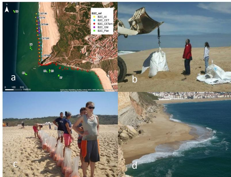
**Fig.2.** (a) Norte beach tracer experiment plan; (b) 12 T collection of native sand; (c) 16 kg shots of fluorescent coated sand for continuous injection (total of 630); (d) Prainha beach formed on the end of the summer nourished by headland sediment bypassing.
