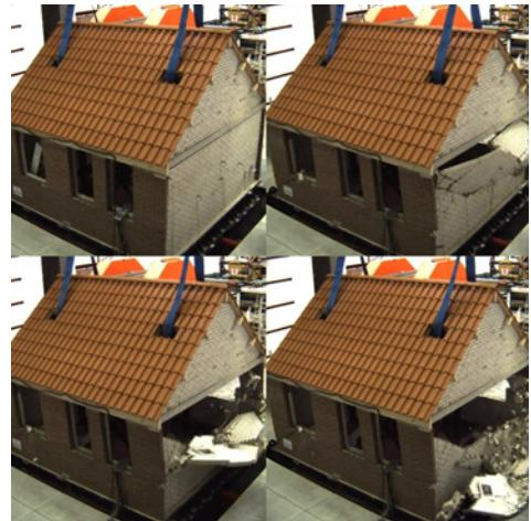
Testing in the LNEC-3D seismic platform of full scale single-family buildings representative of a typical Dutch house with a view to characterise their seismic performance for different intensities of earthquake action.
