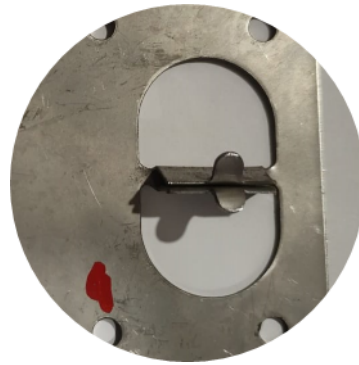
Figure A5.2 – Type of CRM.04-O skin element fixing rupture – vertical load (weight)
