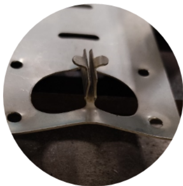
Figure A5.5 – Type of CRM.04-O skin element fixing rupture – horizontal load (wind)
