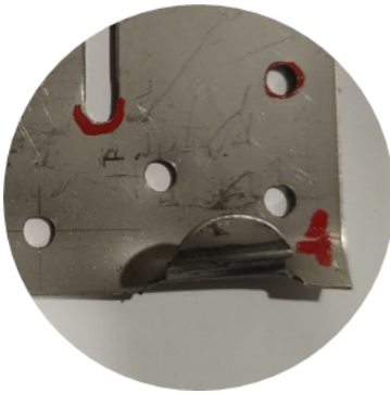
Figure A5.3 – Type of CRM.03 skin element fixing rupture – vertical load (weight)
