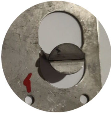
Figure A5.1 – Type of CRM.04 skin element fixing rupture – vertical load (weight)
