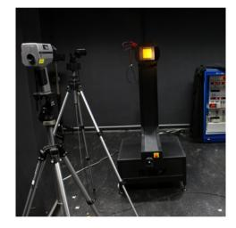
This laboratory also conducts tests for determining the optical characteristics of car components and signalling and hence providing vital support to the Portuguese and international industry
