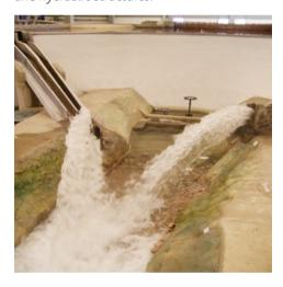
UMEHIF has two testing halls with an area of 5000 m2, which are supplied by hydraulic circuits with a capacity up to 1000 l/s. It is also equipped with high precision equipment for measuring physical magnitudes applied to hydraulics. UMEHIF consists of physical models of hydraulic structures (spillways, intakes, hydraulic circuits, etc.) and ten experimental facilities/flumes.
